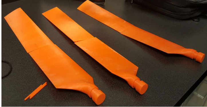
Figure 13: Baseline pin locking mechanism replica of Wind Turbine Technologies turbine blade
